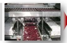
surplus levels of product on the calibration rolls are removed, thus leaving **always only one level** (or row) **of the product on calibration rolls** - the first condition for a perfect calibration
